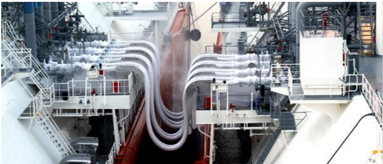
Figure 8: Transfer of LNG from carrier vessel to FSRU using cryogenic hoses.
