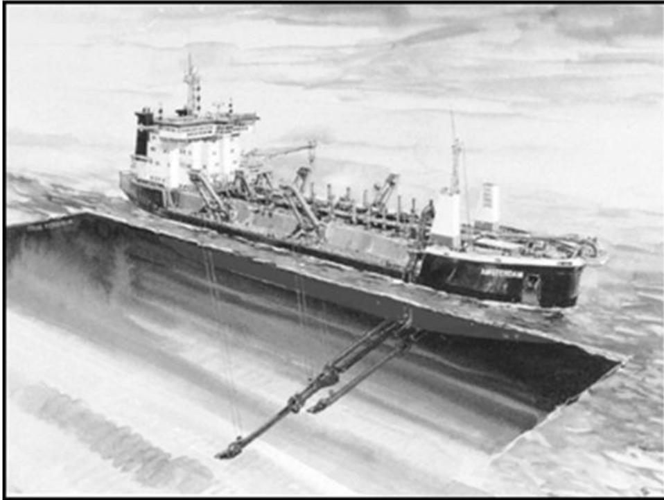
*Figure 2-2: Schematic of a TSHD operating in relatively shallow water.*
