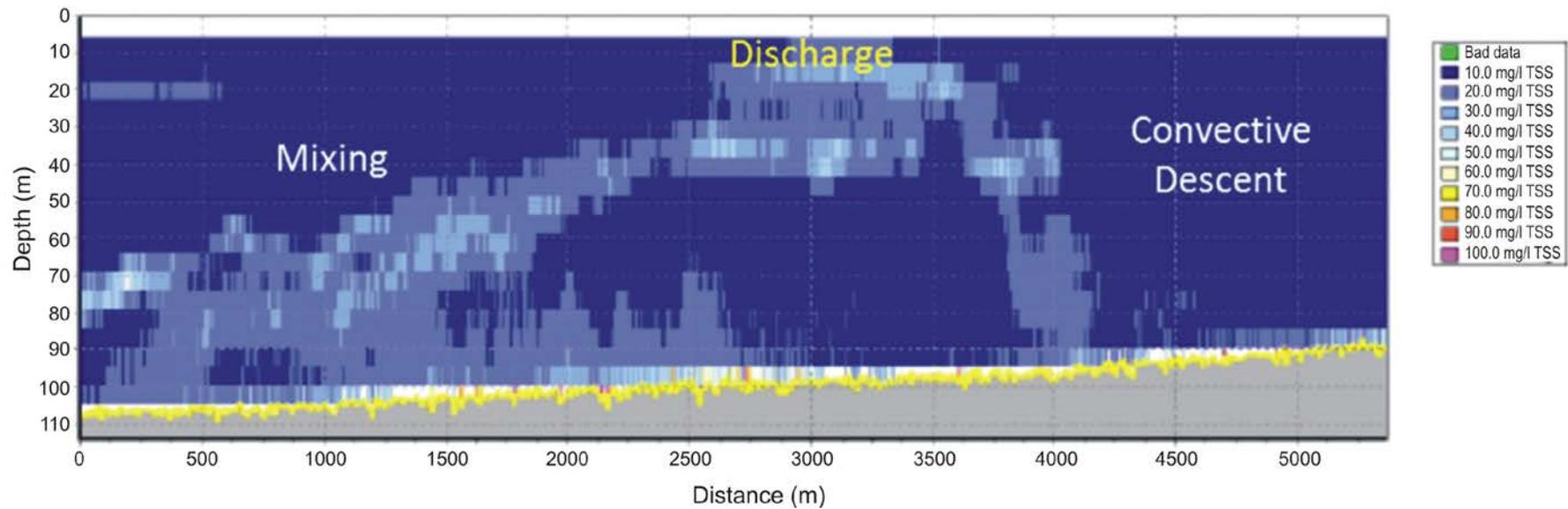
**Figure 4-2: An example of the vertical structure of an overspill discharge plume generated by dredging muddy sand sediments (from CSIR 2006b).**
