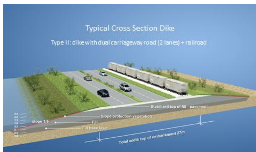
Figure 7: Typical dyke section with dual carriageway
